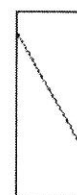
Type 4 Diagonal fracture with no cracking through ends; tap with hammer to distinguish from Type 1
